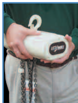
The SLM is about 12" in length, and weighs less than 35 lbs.
